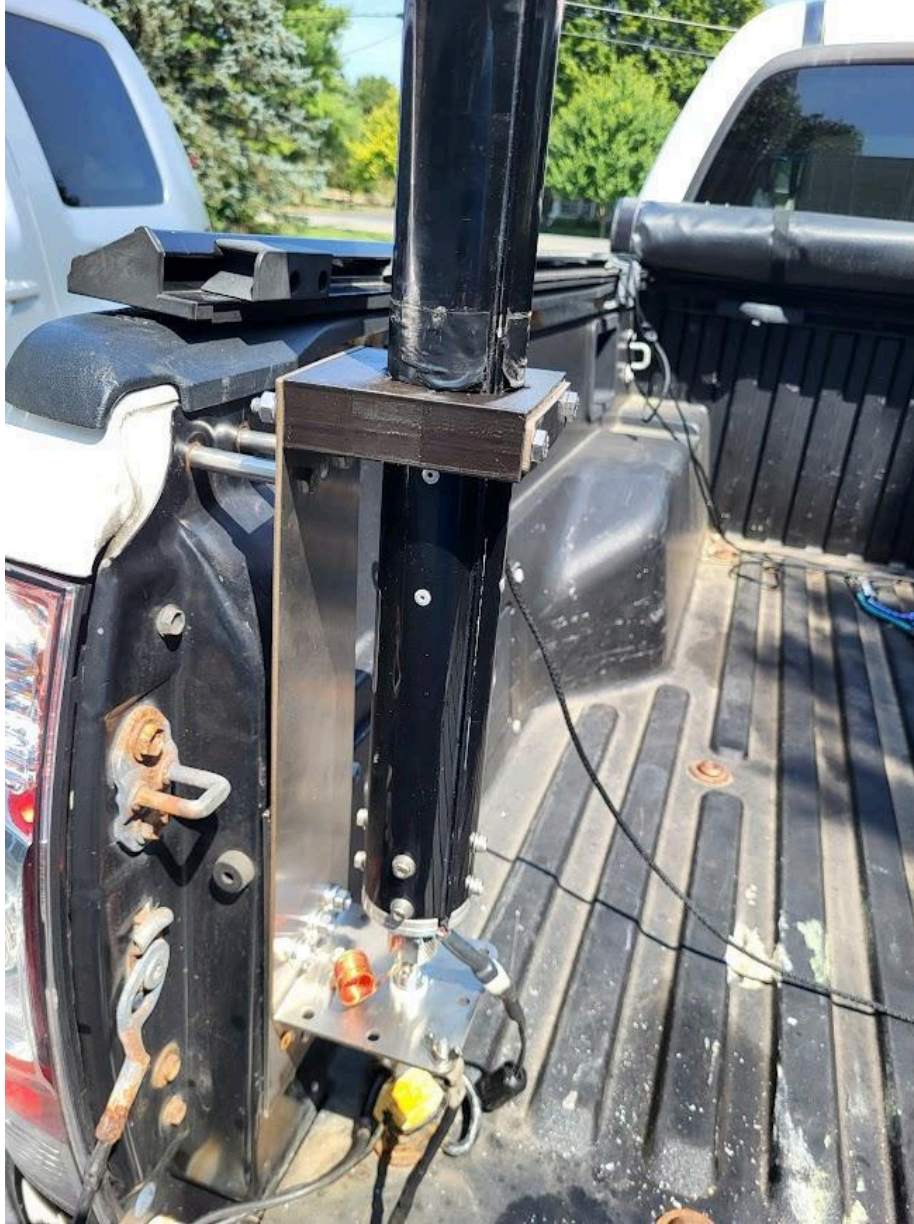
The Tarheel 100HP mounted in the bed of N2B's Toyota Tacoma. (N2BEG photo)
