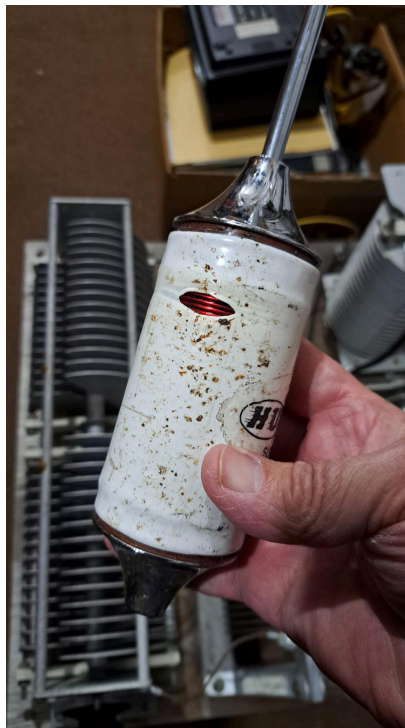
The N2T 40-meter high-power Hustler coil “met its match” with 500 W of CW action in NYQP. At least the vinyl overwrap found its limit! The combination of authentic NYQP bugs and automatic ventilation made for a fantastic after-the-fact photo op. (N5OT photo)
