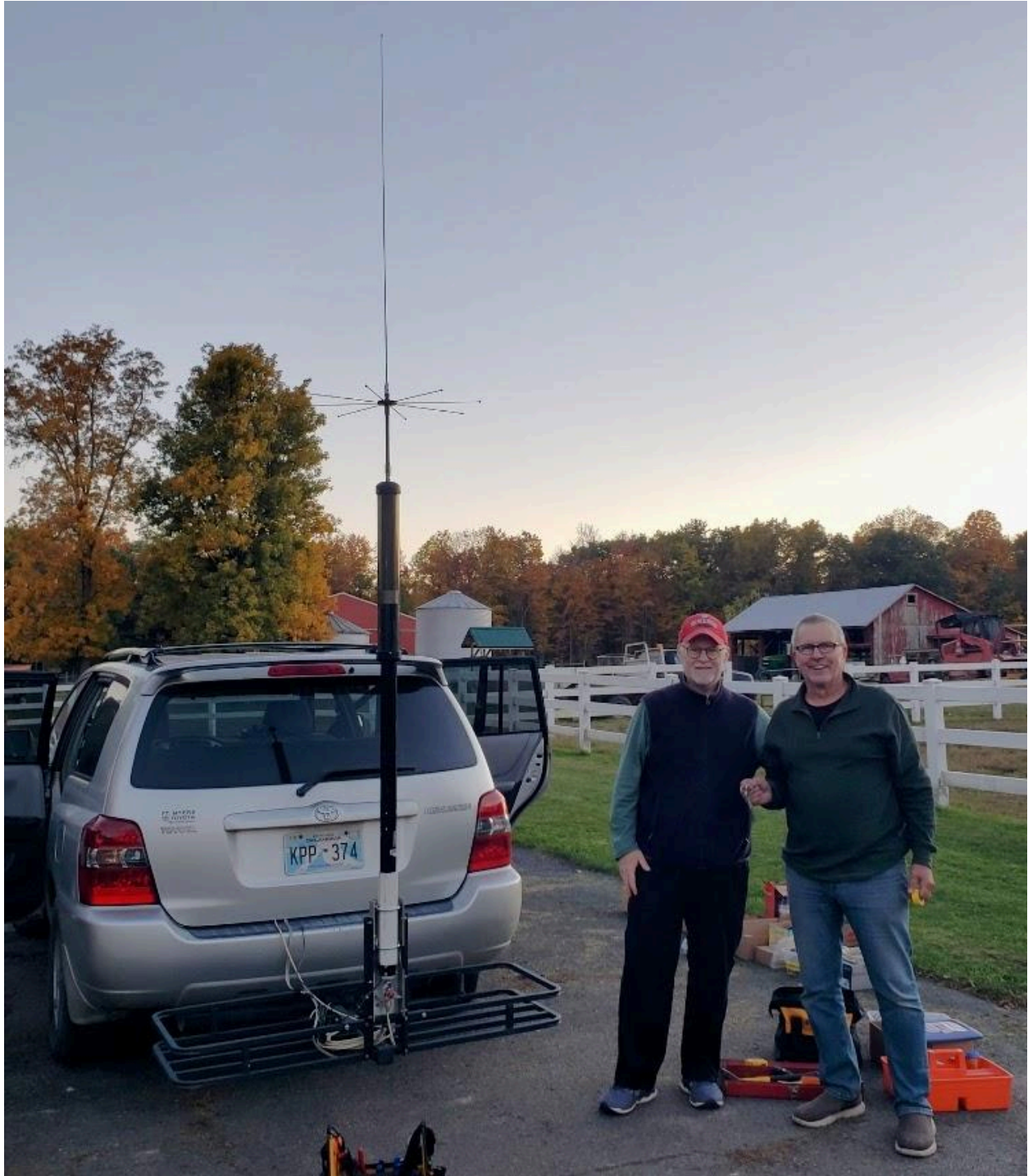
(L-R) K2UA and N5OT celebrate completing the N5OT mobile antenna installation after running through antenna installation on a home-brew mount, cabling, and SWR testing on all the contest bands from 15-80 meters, just as the sun sets on Friday evening before NYQP starts the next morning. (N5OT photo)
