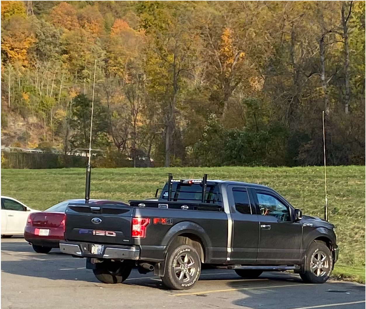
The N2MG/M vehicle, piloted through 22 counties to a 193k score and a win in the multiop mobile CW category by N2ZN and N2MG. A pair of Tarheel 100A-HP antennas adorn the front and rear of the truck, with a TS480HX and SG-500 amplifier inside. (N2ZN photo)
